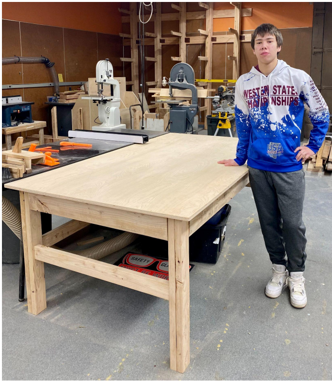
Jordan Leinberger designed and built an outfeed table for the table saw. The table was built using dimensional lumber and 3/4" birch plywood.
