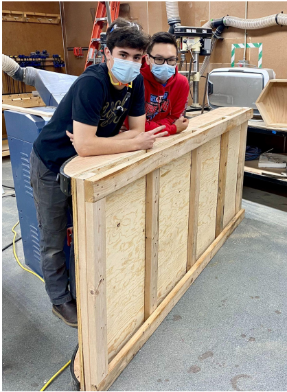
Peter Crow and Tyler Laroux designed and built this wooden sled that they plan to use for logging this winter. The sled is made from dimensional lumber and UHMW for runners.
