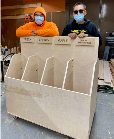
James Bright and Malcolm Queenie designed and built this wood storage bin out of 3/4 birch plywood. They used a pocket hole jig and screws to fasten the pieces together. They also used the laser engraver to make signs for each cubby indicating the various species of wood we use in the woodshop.
