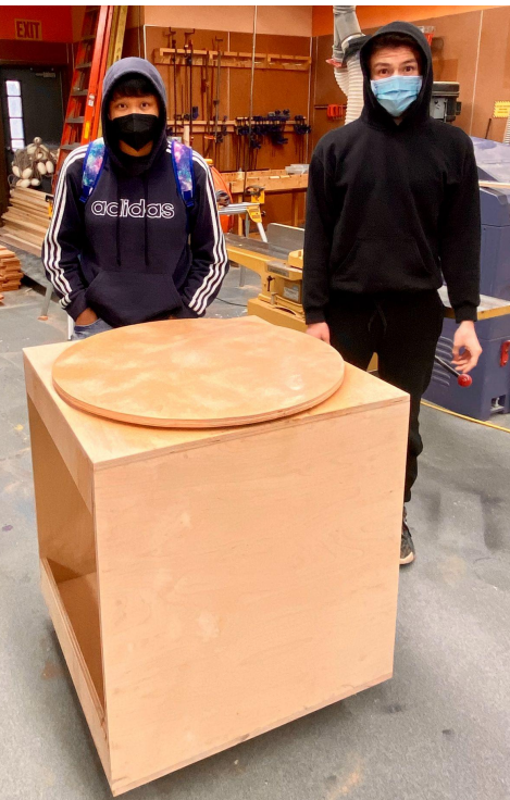
Trinity Chadwick and Jason Kupanoak designed and built this lazy susan spray table using 3/4" birch plywood. They used a pocket hole jig and screws to fasten the pieces together. The top spins to allow the user to spray an even coat of finish on all sides of any project.
